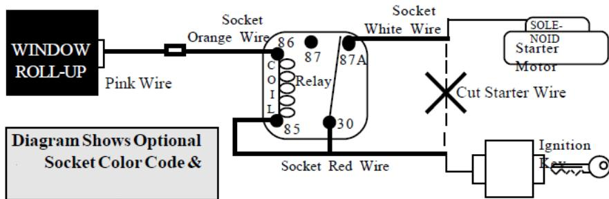
**FUNCTION 2:** To have a relay supply 12 volts positive or ground to other detection devices when alarm is armed activating the WT2.
